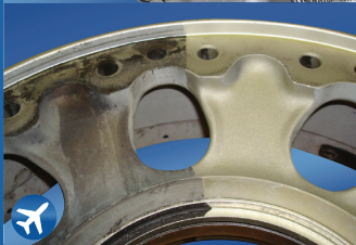
Expose Crack & Prep for LPI
