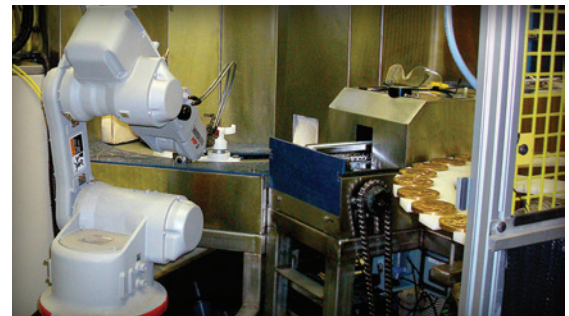
Fully automated, six-axis robotic pick and place system for loading, descaling, rotating, rinsing and unloading commemorative coins. No hazardous acid washes or dust-producing dry blasting. Client: US Mint
