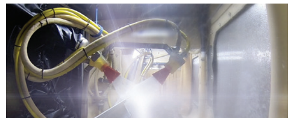
High volume liquid abrasive and high pressure water surface finishing system.
