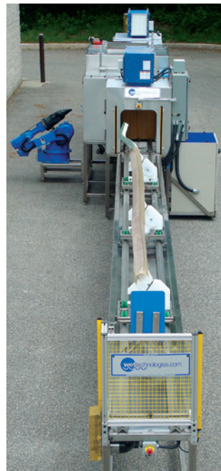
Composite bonding preparation for Helicopter Rotor Blades. Client: Boeing
