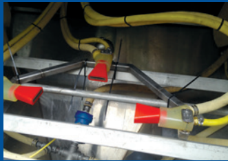
Revolving and rotating nozzles allow for simultaneous finishing of all sides and angles of large and complex parts. Client: Boeing
